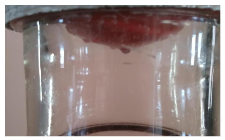
The contraction of the air and water inside the lamp will draw down the red silicone sheet as it creates a vacuum. This is now your new expansion chamber.
