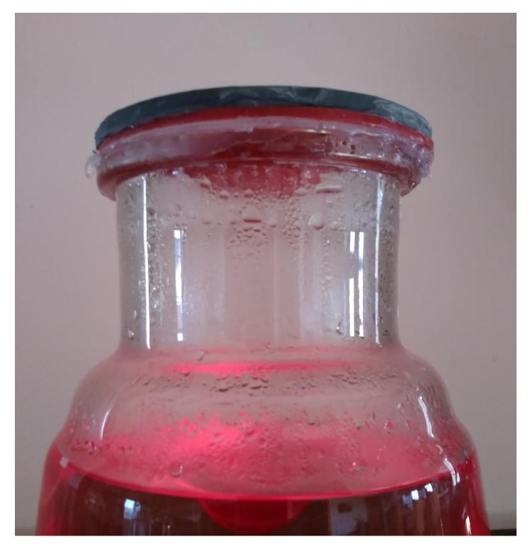
Install your cap.(DO NOT SILICONE IT TO THE RUBBER) To re-crimp the seal, I find it is best to either leave on the old heat shrink around the neck or use layers of masking tape to protect the neck of the globe while tapping down the edge of the cap. I use a small hobby jewelry hammer to tap the rim of the cap back in place.
